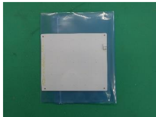
Figure 6. Assembled PCB that is Packed in an Antistatic Bag
