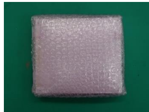
Figure 5. Assembled PCB that is Wrapped with Antistatic Bubble Wrap
